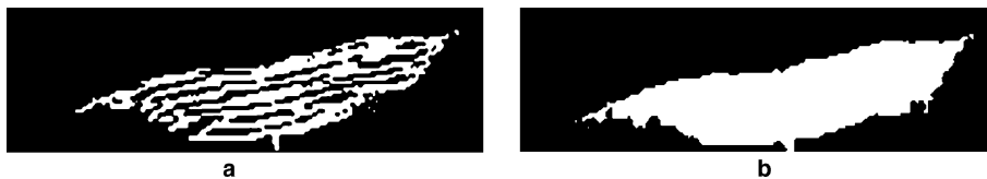
Fig. 3. Example of a fibre section before (a) and after (b) lumen filling.
